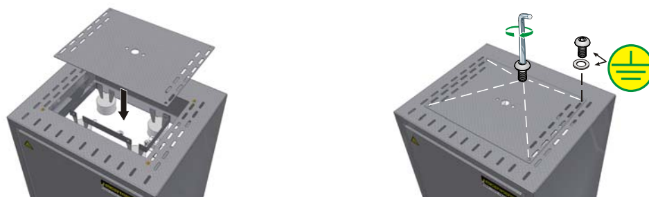
Fig. 32: Installing the furnace lid
